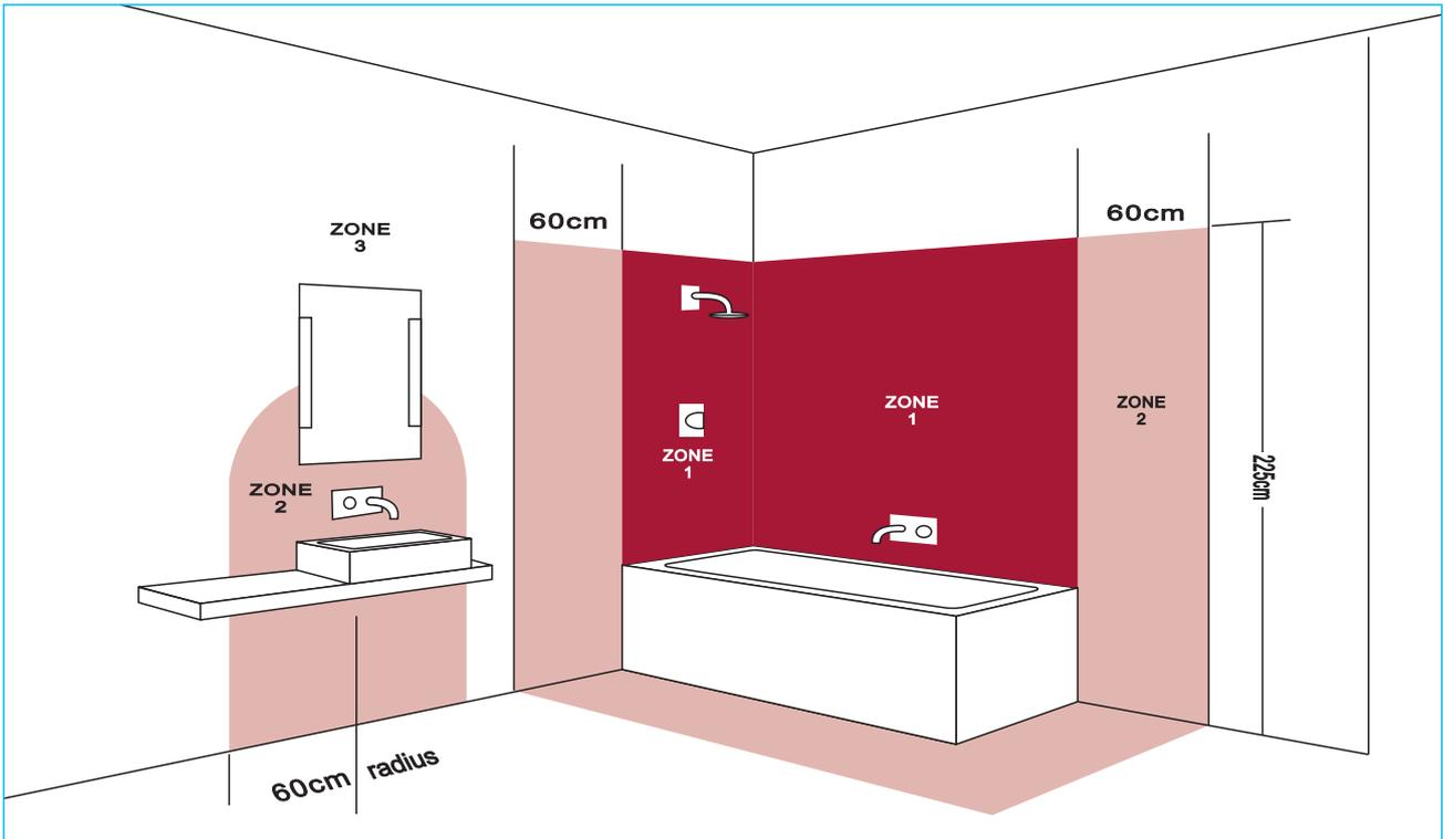
These mirrors are suitable for Zone 2 or higher and not Zone 0 or 1 (see diagram above). (Fig 1)
